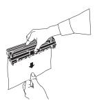
4 Slide the image drum back into place, aligning it under the tabs (a). Press down firmly to lock the drum in place.
