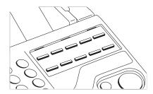
Use the One Touch keys for quick, one-touch dialing. They are also used to access most functions and programming options.
