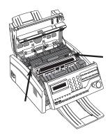
5 Install a new toner cartridge. Follow Steps 3-7 in "Replacing the Toner Cartridge" in this section.
