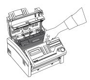
**3** Firmly lift up to disengage the drum cartridge (with its toner cartridge), then lift it out. Wrap it in the packaging materials from your new drum cartridge, and discard it.
